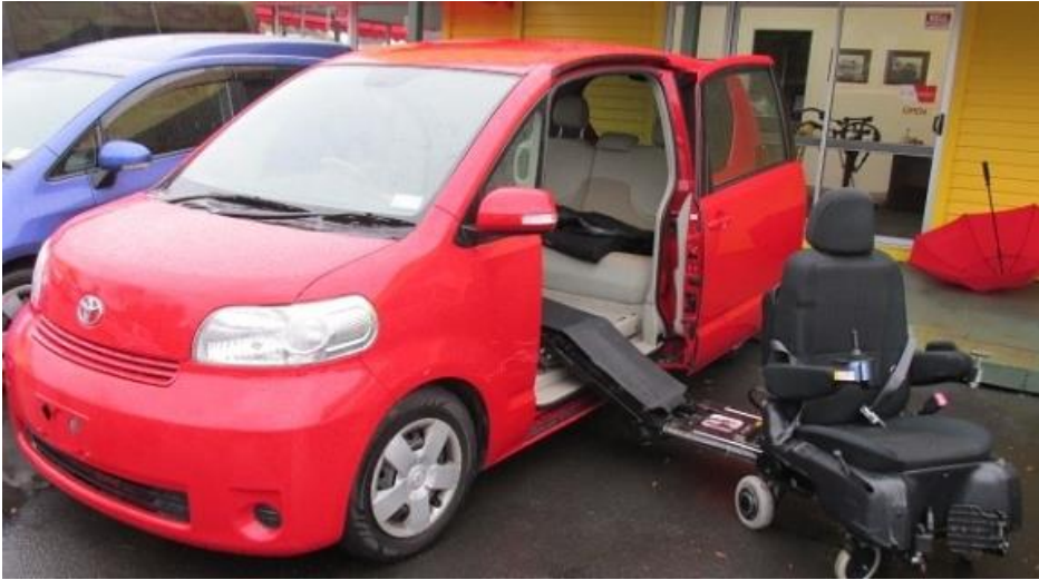
Figure 7-1: 2008 Toyota Porte vehicle with entrance and exit via a portable driver's seat. (Image reprinted from https://www.rodmilner.co.nz/ )
